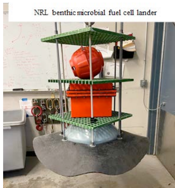
Figure 4-1 Deep Water Sentinel (DWS) fuel cell package.
