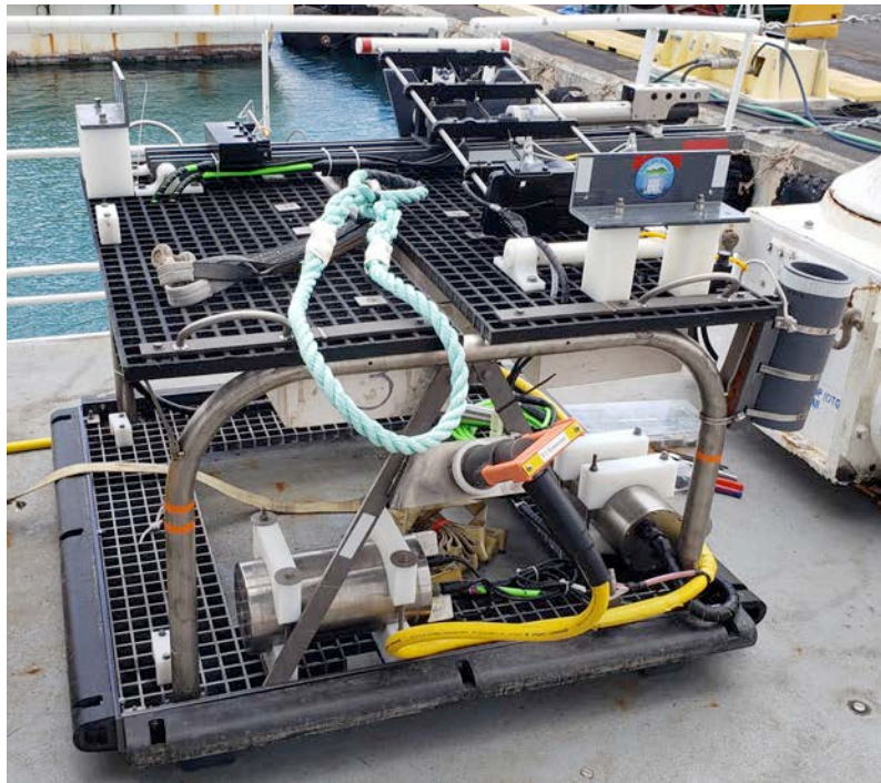
Figure 3-2 BSP4 with CTDO2, FLNTU, RBR pressure, WHOI micromodem, and SIIM.
