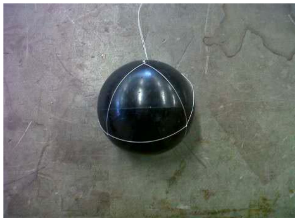
Figure 3-4 Sonar bell passive beacon, 200 mm dia.
