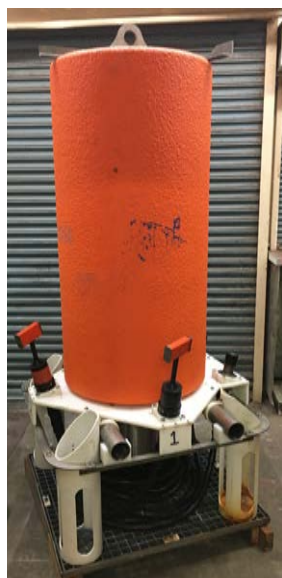
Figure 3-2 BSP3 with cable reel holding 50 m of hose.
