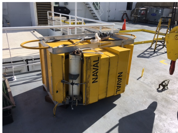
Figure 3-4 Elevator with line basket in front left canister.
