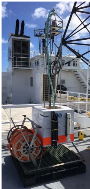
Figure 3-2 BSP3 with cable reel holding 50 m of hose.
