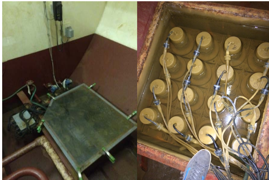
Figure C-1 Housing and interior view of the 4x4 transducer array located on the hull of the R/V Kilo Moana
