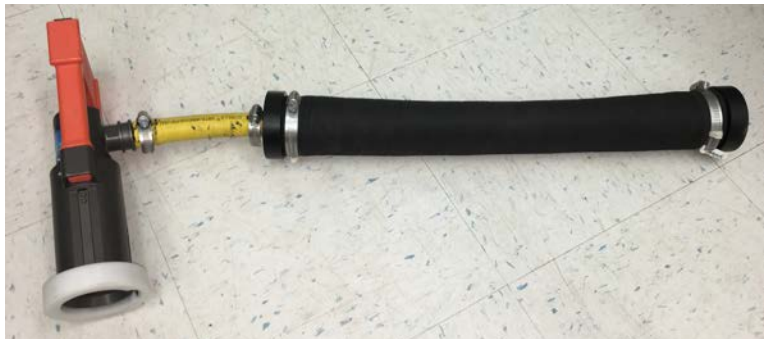
Figure 9-1 Power load test tool
