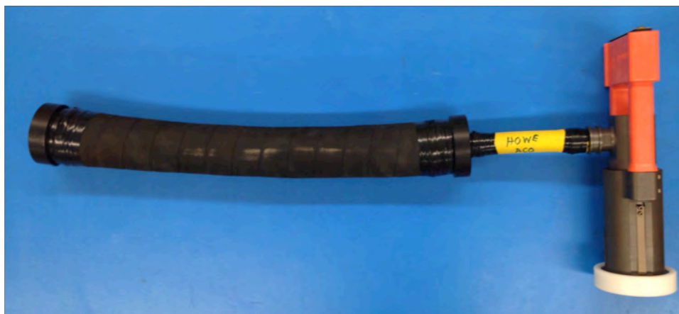
Figure 3-11 ACO port test tool
